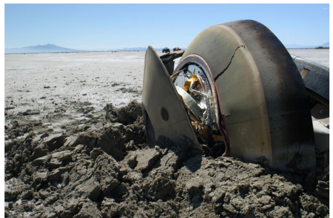
Fig. 5. Closeup view of the damaged Genesis capsule after its return to Earth. NASA/JPL-Caltech.
