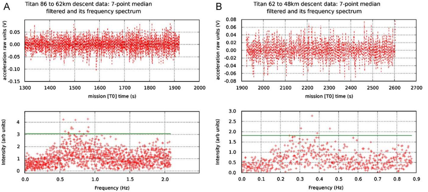
**Fig. 15.** (A) Frequency spectra from the probe's descent under the drogue parachute. While the descent from 86 to 62 km (Fig. 15(A)) show dominant frequency components around the modelled oscillation frequency of 0.8 Hz (in Fig. 14), the latter part of the descent: from 62 to 48 km (Fig. 15(B)), shows no evidence of the modelled frequency.
