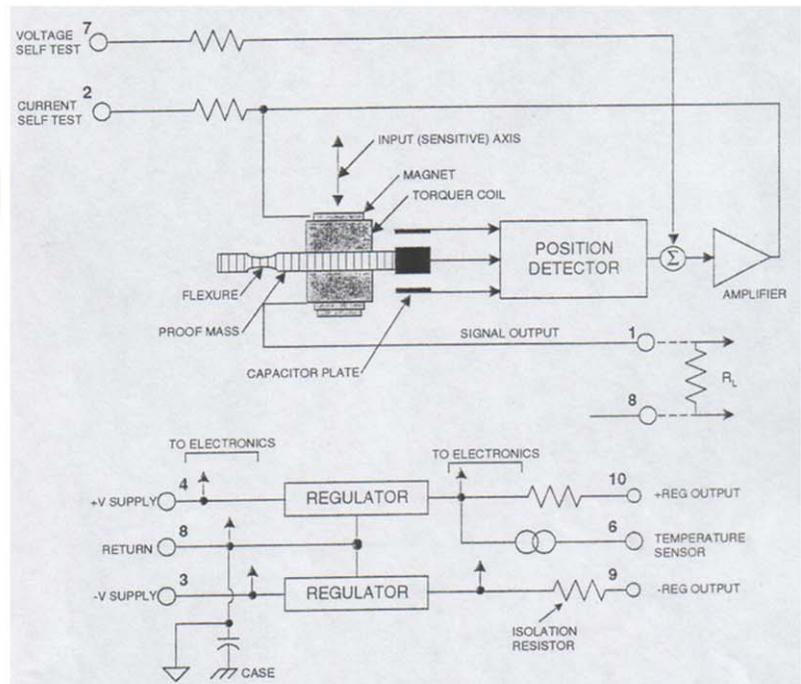
**Fig. 2.** The Servo sensor (QA2000, Q-Flex accelerometer), along with its main properties. The right-hand section of the image shows the schematic representation of the Servo unit. The voltage across resistor  $R_L$  gives a measure of the acceleration;  $R_L$  also determines the device's sensitivity in terms of volts per unit acceleration (V/g). The device has an inbuilt temperature sensor.
