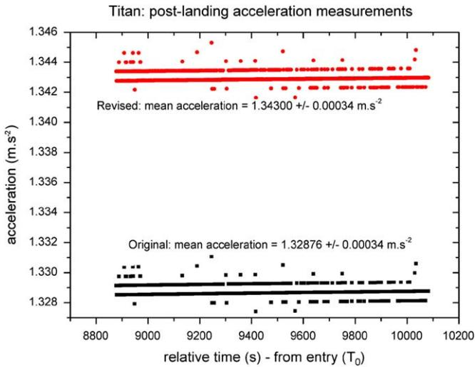
**Fig. 16.** Post-landing acceleration measurements (on Titan's surface) show the revised values to be higher by about 1% than original values. The revised value, calculated by taking the offset drift during cruise into account, is closer to the Titan's reference gravity of  $1.345 \text{ m.s}^{-2}$ , quoted in Lebreton and Matson (2002).
