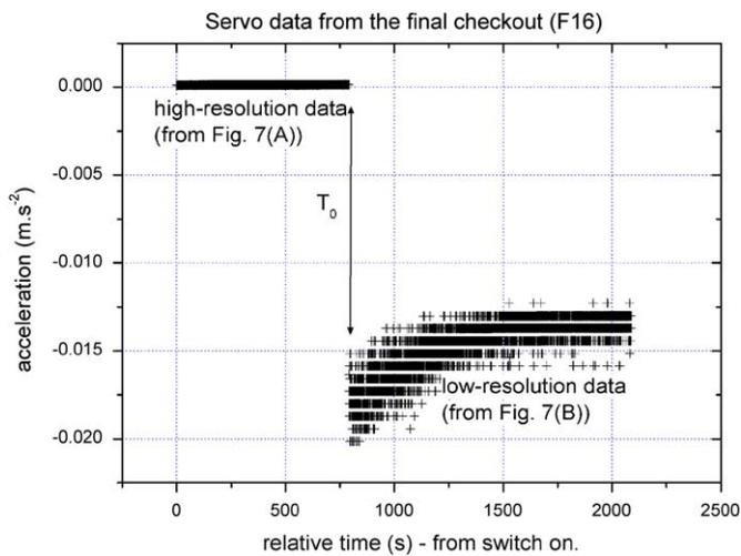
**Fig. 11.** When converted using the information from Appendix A, the high-resolution entry and the low-resolution descent data do not 'line-up' as they should given the constant (0 g) acceleration. This step in the two data sets from the same cruise checkout demonstrates the need to adjust the Servo's offset according to its measurement range as well as its operating time and temperature.
