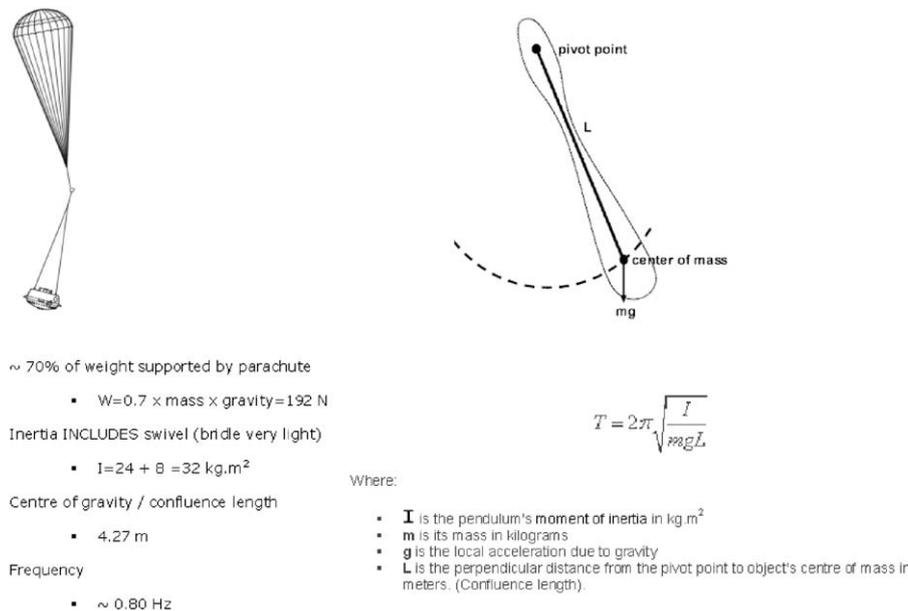
**Fig. 14.** Schematic of the Huygens probe under stabiliser chute (left), and the parachute model (right). Oscillations due to the faster 'half-scissors' swing mode should be around 0.8 Hz, while the slower 'rigid-pendulum' mode, with length of 12 m should be around 0.05 Hz (i.e. period = 20 s). The parachute calculations and details are available in Underwood et al. (2005).
