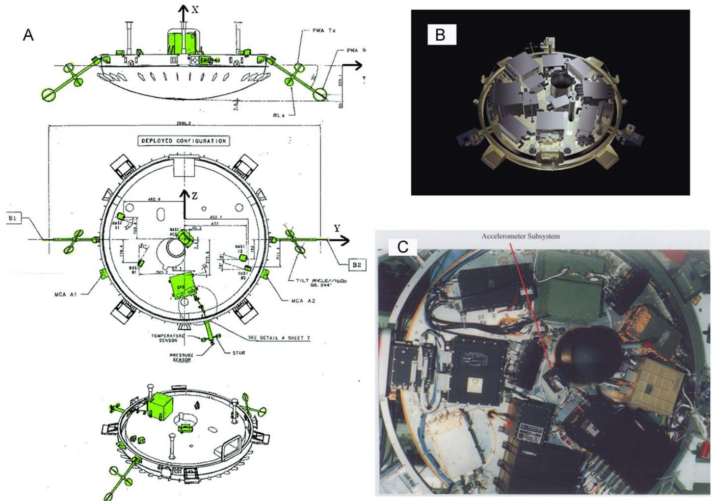
**Fig. 1.** Shows the central location of the accelerometer sub-system unit, containing the Servo, from the technical drawing perspective (A), the computer-aided-design CAD (B), and the photograph (C). The HASI Servo is located as close to the Huygens probe's centre of mass (CM) as possible; its location relative to the CM, in the probe's reference frame  $[X, Y, Z]$ , is  $[-6.00, 14.65, 1.42]$  mm (Colombatti et al., 2008b).
