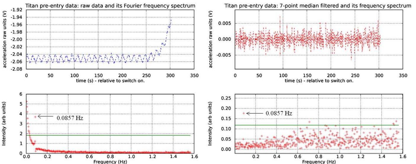
**Fig. 12.** Servo data prior to the atmosphere encounter and its frequency spectrum. The top-left figure shows atmosphere detection at the tail end of the plot. The dominant frequency component (at 0.086 Hz), along with other probe dynamics-related information, has been used to calculate the spin rate of  $\sim 7 \text{ rpm}$  (Colombatti et al., 2008a).
