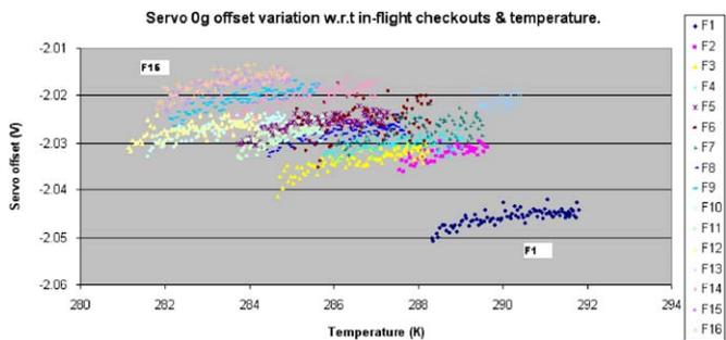
**Fig. 10.** Variation in the offsets from the high-resolution (up to  $\pm 2\text{mg}$  or  $\sim \pm 0.02\text{ m s}^{-2}$ ) data from all cruise checkouts. These raw values must equate, on average, to zero acceleration. Hence, the cruise measurements are useful in obtaining the zero-g offset values (used in Eq. (2)). We see a small drift the Servo’s offset ‘upwards’ on the plot over time (i.e. moving to less negative values).
