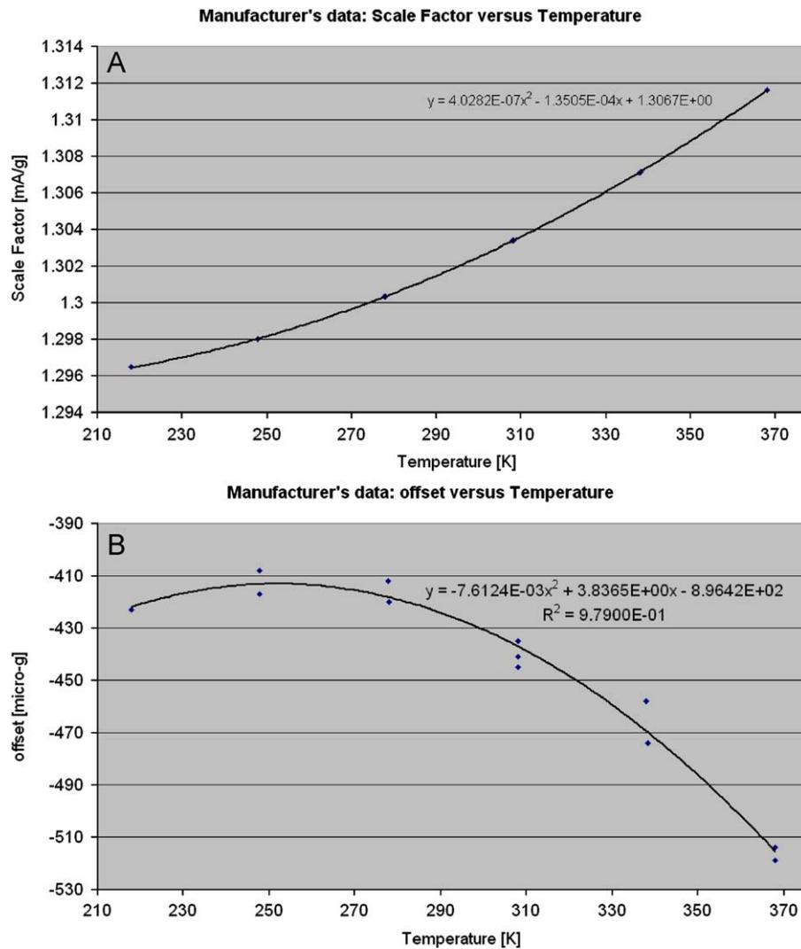
**Fig. 17.** (A) Servo's scale factor as a function of temperature from manufacturer's calibration of the specific flight sensor. Changes to these values over time have not been monitored. (B): Servo's offset as a function of temperature from manufacturer's calibration of the specific flight sensor. These values can be monitored during cruise/ in-flight checkouts.
