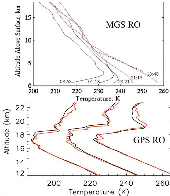
**Fig. 2. a.** Diurnal changes in lower atmosphere thermal structure in between  $30^{\circ}\text{S}$  and  $60^{\circ}\text{S}$  seen in MGS RO (radio occultation) measurements (Hinson et al. 1999). **b.** Comparison of close-coincidence GPS RO and balloon profiles in Earth's tropics near the transition between the troposphere and stratosphere demonstrating the vertical resolution of GPS occultations. Black: GPS, Red: balloon. The two profiles to the right are offset by 20 K each.
