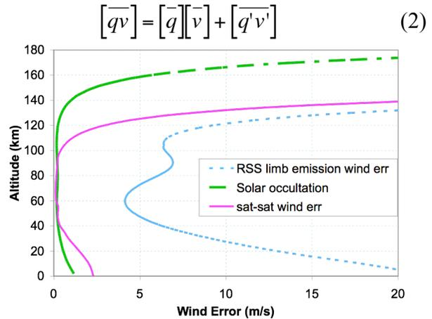
**Fig. 3: Accuracy of individual mm-wave Doppler wind measurements for sat-sat RO, SO and TE profiles. Accuracy improves further with averaging.**
