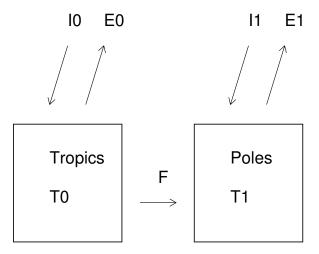
Figure 10.1: Simple two-box climate model. The boxes are of equal surface area, the left (subscript "0") corresponding to regions equatorward of  $30^{\circ}$  latitude and the right (subscript "1") to regions poleward of  $30^{\circ}$  latitude. I is absorbed solar flux, E is outgoing thermal flux, and F is the rate of latitudinal heat flow per unit area. T is temperature.
