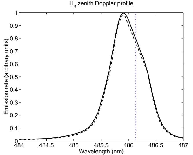
**Fig. 6.** Modelled  $H_{\beta}$  line profile along the magnetic zenith, including angular redistribution in the transport of the precipitating  $H/H^+$  stream. The dashed line shows the theoretical line profile, the solid line is the same profile after convolution with the HiTIES instrument function. The rest wavelength is indicated by the dotted line.
