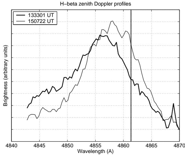
**Fig. 5.** Spectrum of the  $H_{\beta}$  line spatially integrated over  $\phi^{\circ}$  in the magnetic zenith at 13:33:01 UT and 15:07:22 UT. The background brightness is subtracted. The unshifted wavelength is at 4861.3 Å. The blue shifted component results from the line of sight velocity of downward moving hydrogen. The red shifted wing is the consequence of upward moving hydrogen.
