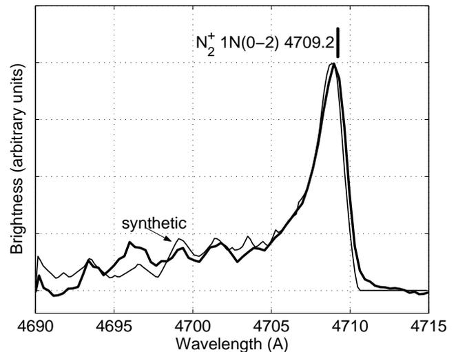
**Fig. 4.** Spectrum of the spectral window (magnetic zenith) for  $N_2^+ 1N$  ( $4709 \text{ \AA}$ ) integrated from 13:00-14:20 UT. A synthetic spectrum of  $N_2^+ 1N$  with neutral temperature of 1500 K is superimposed.
