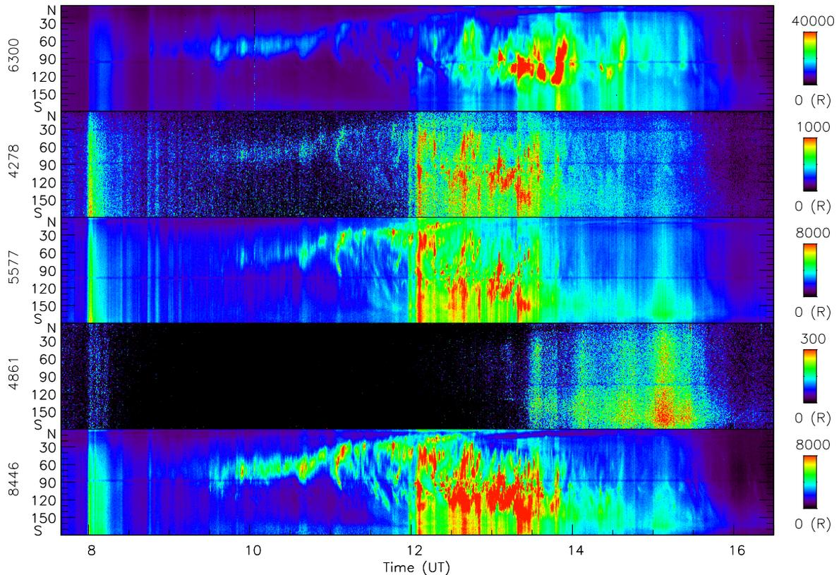
**Fig. 2.** Data from the Svalbard Meridian Scanning Photometers. Each panel shows the auroral brightness as a function of meridian scan angle and time. The wavelengths shown are (top to bottom) OI(6300 Å),  $N_2^+$  1N(4278 Å), OI(5577 Å)  $H_\beta$ (4861 Å), OI(8446 Å).
