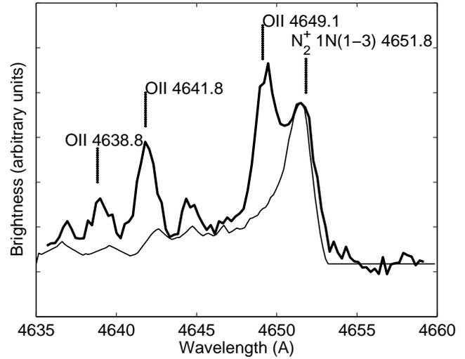
**Fig. 3.** Spectrum from the HiTIES instrument (magnetic zenith) integrated from 13:00-14:20 UT. Auroral emission features are indicated. A synthetic spectrum of  $N_2^+ 1N$  with neutral temperature of 1500 K (thin line) is superimposed.
